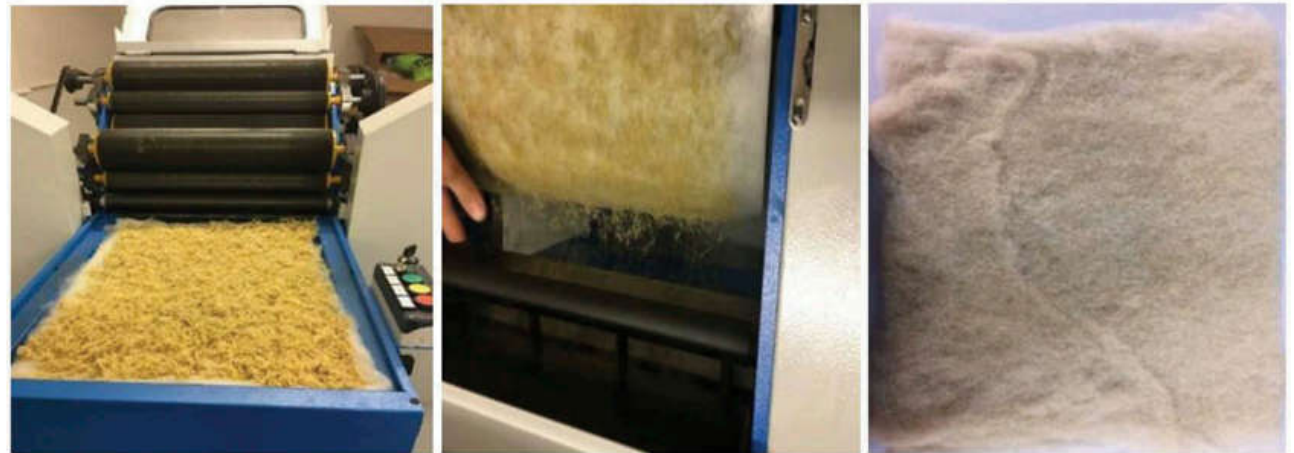
Figure 3. Laboratory-type carding machine and carding band made of rice straw fibers.
